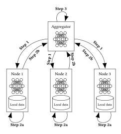
Figure 1: Typical training process of a horizontal Federated Learning system.
